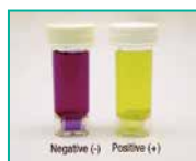
CC-109 Coliform Medium 9 mL (AOAC-RI) Product Specifications Testing time: 4-24 hours Tests per kit: 100
